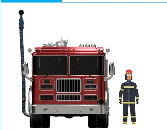
Source capture proactively captures the exhaust discharged from the tailpipe and removes it from the building virtually eliminating exposure to the firefighters.
